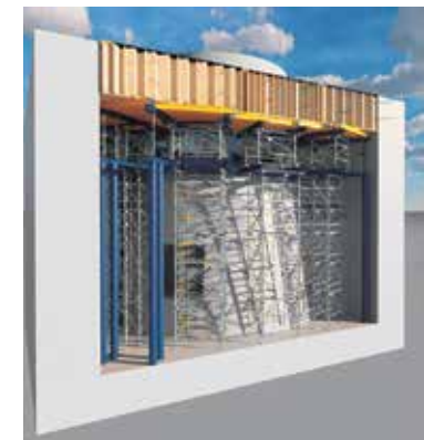
3 Due to the complex geometries of the turbines and inlet slabs, formwork planning would not have been possible without a comprehensive 3D model.
